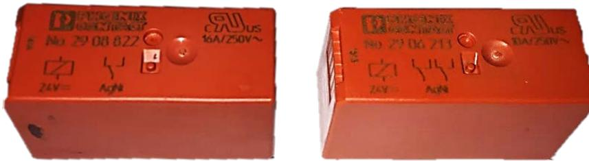
The relay cartridge on the left is Altronic part number 1002-4177-00. It is a 10-AMP relay, SPDT. This relay can only be used on the PR1 (Air Fuel Ratio) socket on the PCB or on a special green relay base.
